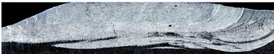
Figure 1 - The microstructure of the sprayed layer at a magnification of 10 times.
