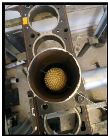
Fig. 2. Ball with golf surface on the purge stand
