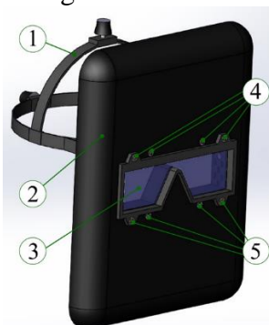
1 - headband, 2 - shield, 3 - protective glass, 4 - upper row of fixing screws, 5 - lower row of fixing screws.
